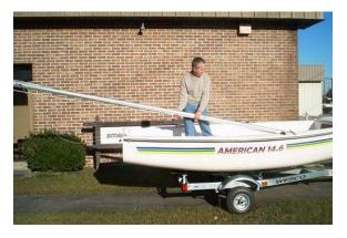
1) Insert the foot of the mast into the tabernacle casting (mast step).
