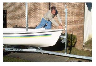
6) Install the forestay into the forward hole in the stem plate, maintaining tension on the mast.
